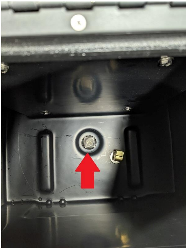
(Ninja 200 freshwater tank acorn strainer and bypass return)
