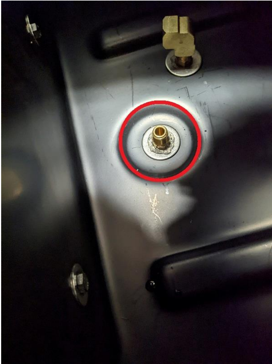
(Ninja 200 freshwater tank acorn strainer removed and bypass return)
