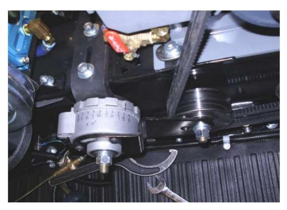
DO NOT over tighten blower belts past the 80 degree (Number 8 mark) mark. If you find that the belts are still too lose after tightening the belts with the instructions above, you may have belts that are either a) the wrong size, or b) stretched out and in need of replacement.
