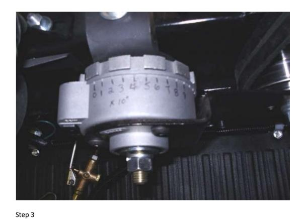
Insert the tensioner tool between the floor and the tensioner with the curved side of the tool facing up and latch the tip of the tool into a grooved slot on the rear of the tensioner plate. (See picture below)
